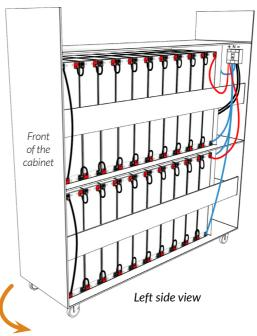
Make sure the cables are correctly connected on each side, then slide the top lid back on and secure it in place.
