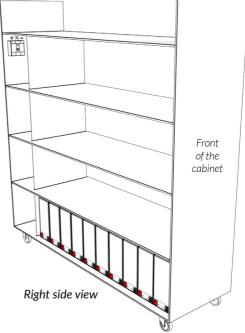
4.2 On the same tray, through the left side, place another set of 10 batteries, vertically, with the terminals facing outwards and down.
