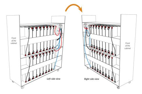
B If you want to use only one string of batteries ( $(16 + 16) \times 1$ ,  $(17 + 17) \times 1$ ,  $(18 + 18) \times 1$ ,  $(19 + 19) \times 1$ ,  $(20 + 20) \times 1$ ), please populate only the first two trays with batteries and follow the same steps for connecting the cables. You will be using only one black cable, one red cable and two blue cables connected to battery cabinet.
