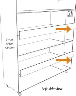
Find the first tray, second tray, third tray and fourth tray on which to place the batteries, as shown on the side picture. Place the batteries starting with the first tray and continue up on the respective trays in a total maximum of 80 pcs.
